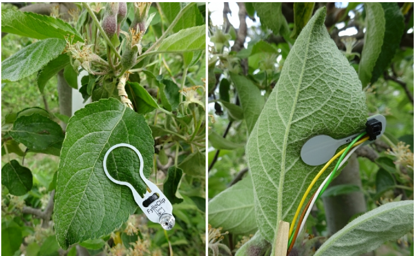
Fig. 1: Front and back view of a FylloClip sensor applied on an apple leaf.
